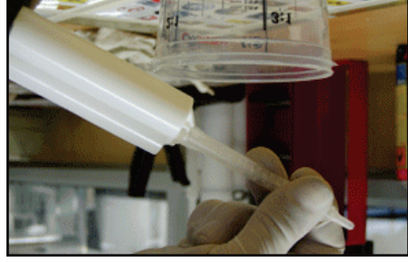
6 Gently break off the seal of the cartridge. Keep the seal in a safe place for resealing later.
