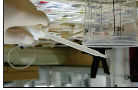
7 Squeeze the dispenser until both cylinders are ejecting resin.
