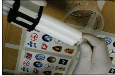
5 Remove the safety cap from the cartridge by turning 90° and gently pulling.
