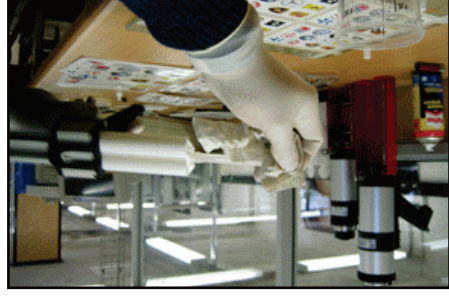
8 Now attached the static mixer to the cartridge. (This screws in)
