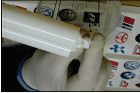
6 Gently break off the seal of the cartridge. Keep the seal in a safe place for resealing later.
